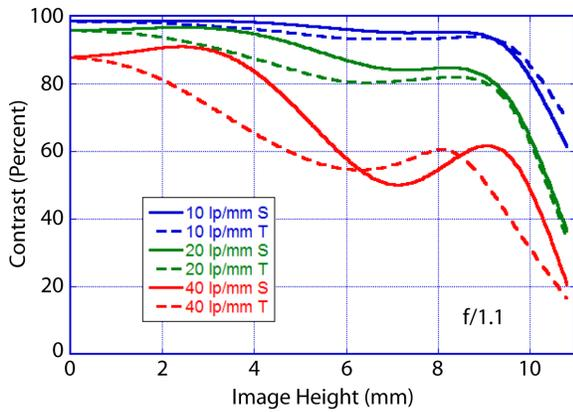
Figure 3: MTF at 10, 20 and 40 lp/mm for f/1.1
