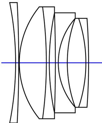
Figure 1: Speed Booster XL 0.64x design layout
